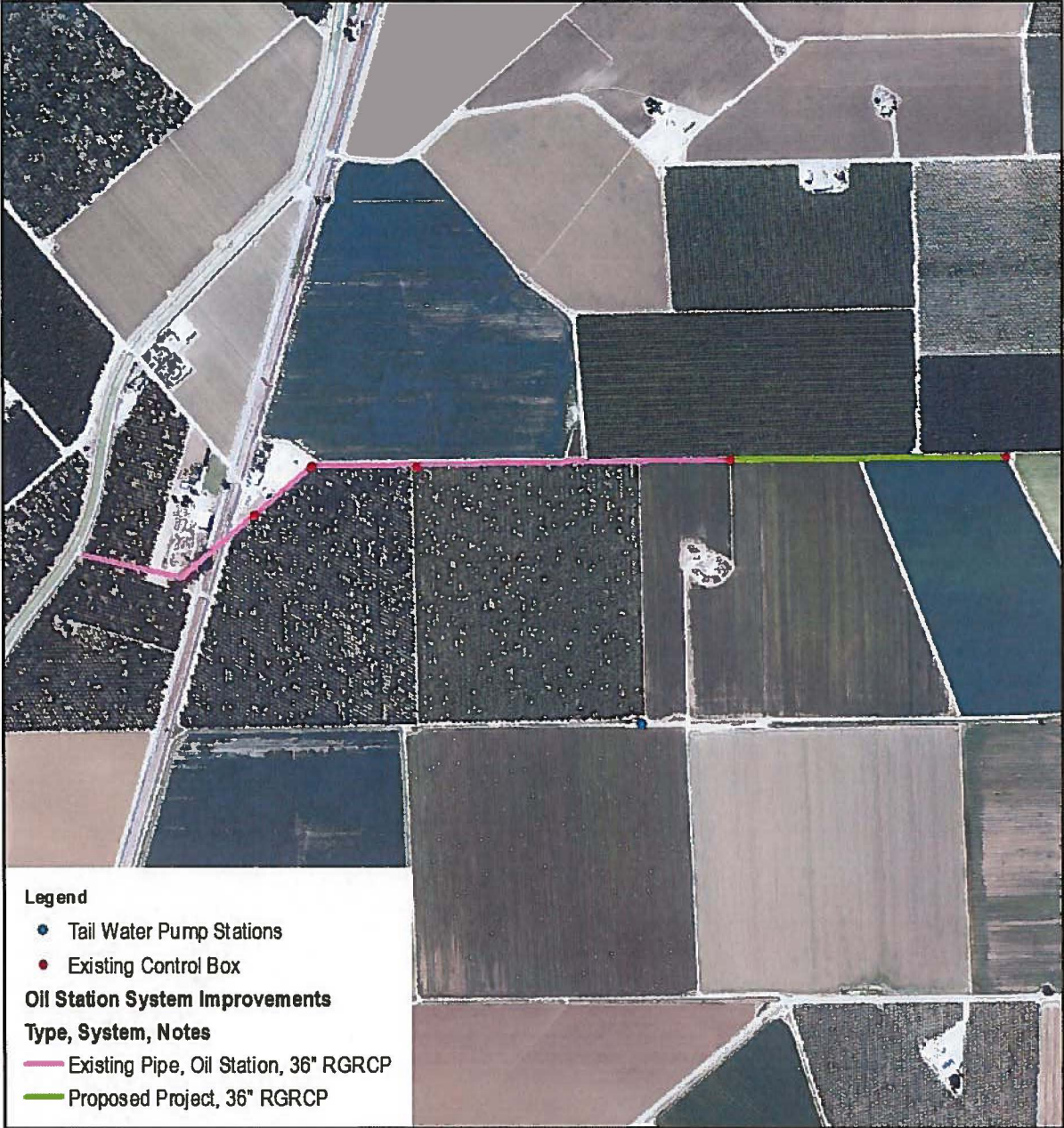
Figure 2: Oil Station Improvements Project Aerial View
